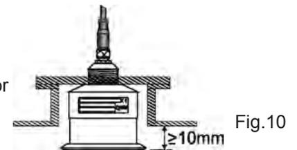
**PTU50-51-56** can be installed in an extension pipe (see Figure 11) to turn away the sensor from the maximum level point. The extension pipe must be flat and without joints (welds, etc..), also, the pipe terminal part must be cut at 45° and with the borders without burr.
