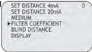
Use **↓** and **↑** to modify the value. Input a value from 1 to 99. Press **OK** to confirm.
