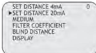
Use **↓** and **↑** to modify that value; in the Fig.22 example, the 20mA distance is 500mm. Press **OK** to confirm.
