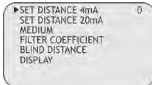
Use **↓** and **↑** to modify that value; in the Fig.22 example, the 4mA distance is 3500mm. Press **OK** to confirm.
