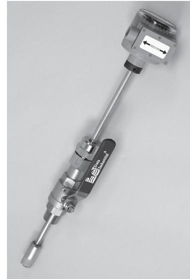
produce an isolated solid state contact closure scaled to any number of engineering units of measure. Sensors may be pre-programmed at the factory or field programmed using a Data Industrial connection cable and a Windows® based software program. All information is stored in non-volatile memory in the flow sensor. This is a four-wire option.
